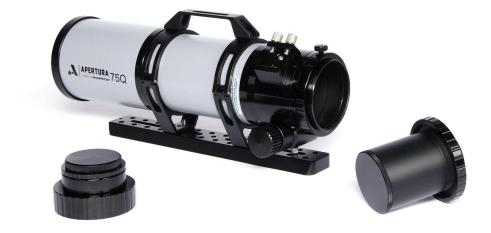
Remove all of the adapters from the focuser just behind the camera rotator.
